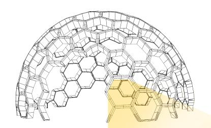
Maryams design will consist of a repetitive replication of a single module mould. Joints will be installed on each corner of the module to then allow a collection of modules to be connected together to create the hallow spherical dome displayed in the above diagram.
