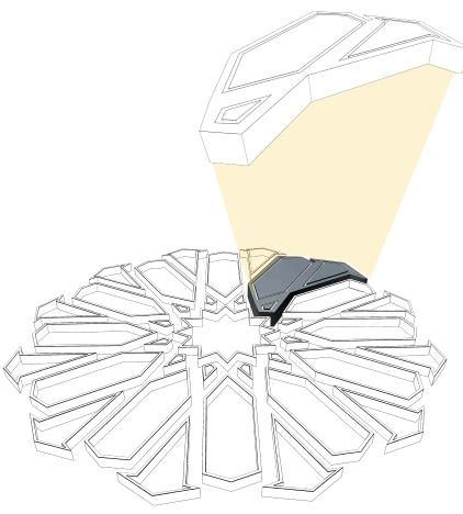
This is the largest proposed design which creates a dynamic space which promotes interactivity and exploration to the user. The symbolic maze stretches a large surface area with a length and width of 60 m and a height of 5.5m, with passageways that are 2m wide for the user to access.
