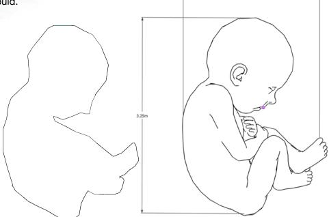
For this proposal, the design of the baby encased in the spherical pattern will be a solid body with complete infill. As an option, the shape could be hallow with a 50mm thickness to conserve material use and reduce weight for ease of transportation to site and installation phase.
