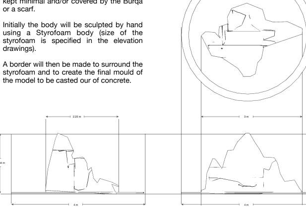
Due to the detailed of the text surrounding the body. The text will need to be CNCed in 3 sections to create the mould which is assembled to create the complete circle of text surrounding the body.
